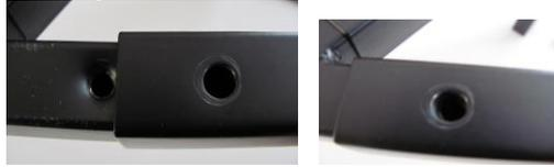
2. Insert screw into hole, initially threading the screw by hand and then tighten with the Allen Wrench so that arms are on securely. \*Do not over tighten\*
